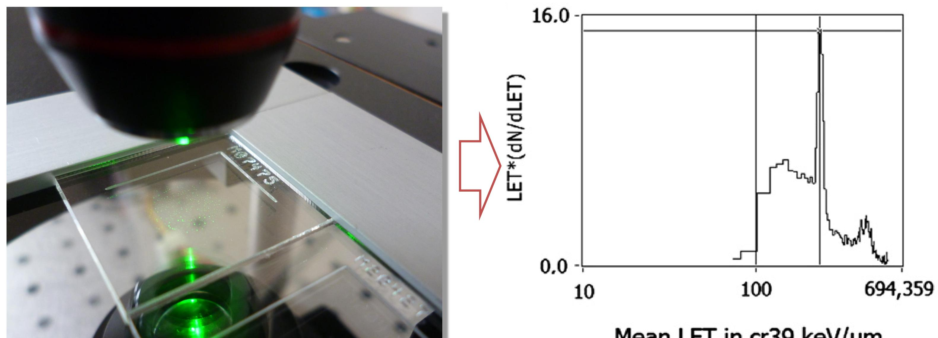
Fig 4. Mean LET distribution of particles impinging on the track detector from the POLITRACK™ SSNTD automatic detector reader.
